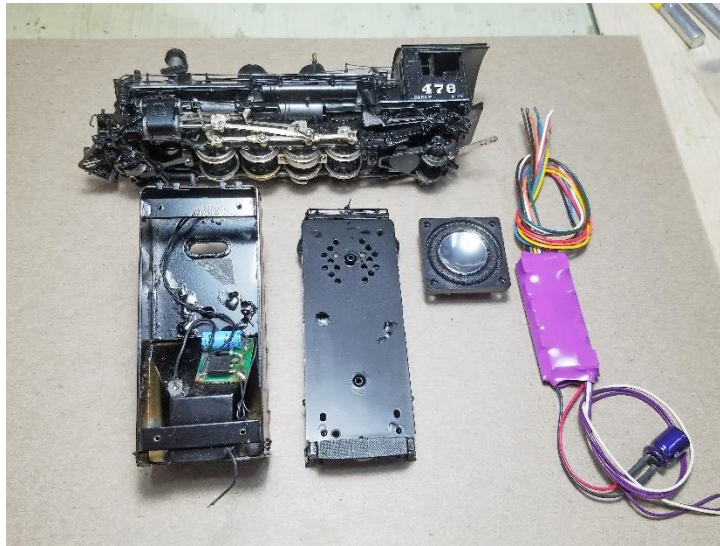
Photo 2: The original installation plan called for using a Tsunami 1 st generation decoder and a 1" square mega bass speaker – but only with major surgery to the tender would these components fit. Switch to Plan B.
