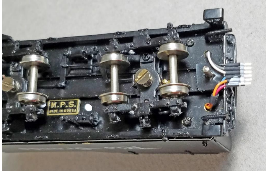
Photo 7: The male end of the 6-pin connector and the 6 conductors were fed through the two holes in the underside of the tender (shown after reassembly of the tender).
