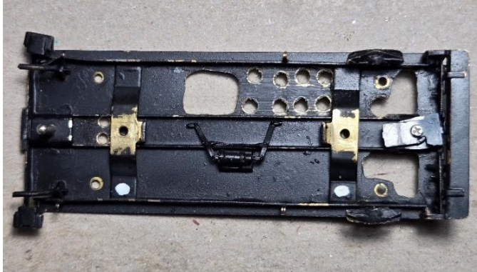
Photo 5: The underside of the tender, with 8 holes for the speaker drilled on the engineer's side and two holes drilled through the center beam immediately forward of the front truck screw hole, at the left. The 3 large openings had been cut out previously for the earlier installed analog system and speaker.
