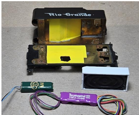
Photos 3 and 4: The three main components, the Keep Alive (green), Tsunami 2 decoder (purple), and speaker (black in a white styrene enclosure) appeared to be a tight fit in the tender, so the sloped sheet (brass) was removed with the help of a jeweler's saw.
